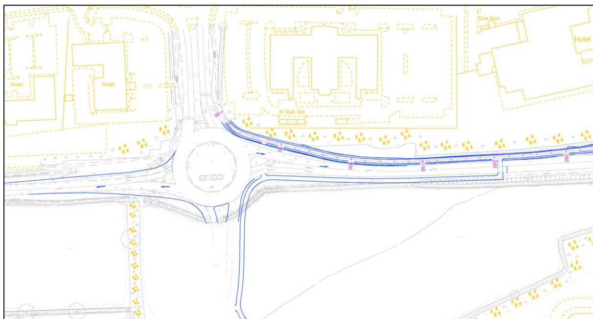
Figure 2.6: A453 EMGP2 Access Junction and Toucan Crossing
